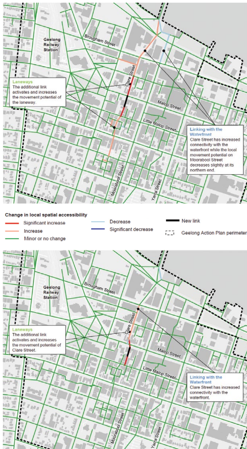
Figure 22. Comparison of the connectivity potential of Dennys Place and McLarty Place. (Source: Space Syntax Limited).
