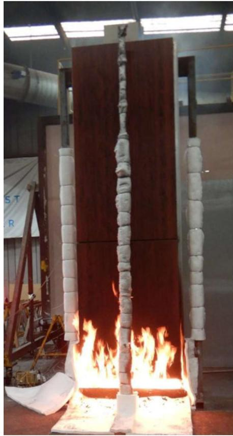
Figure 14 The specimen 8 minutes 49 seconds into the test (burner output at 100 kW)
