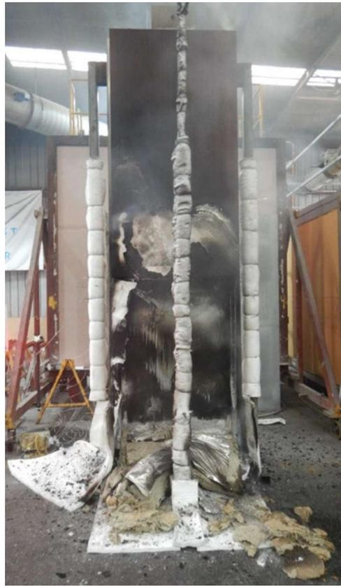
**Figure 26** The specimen after the test, after being sprayed with water.
