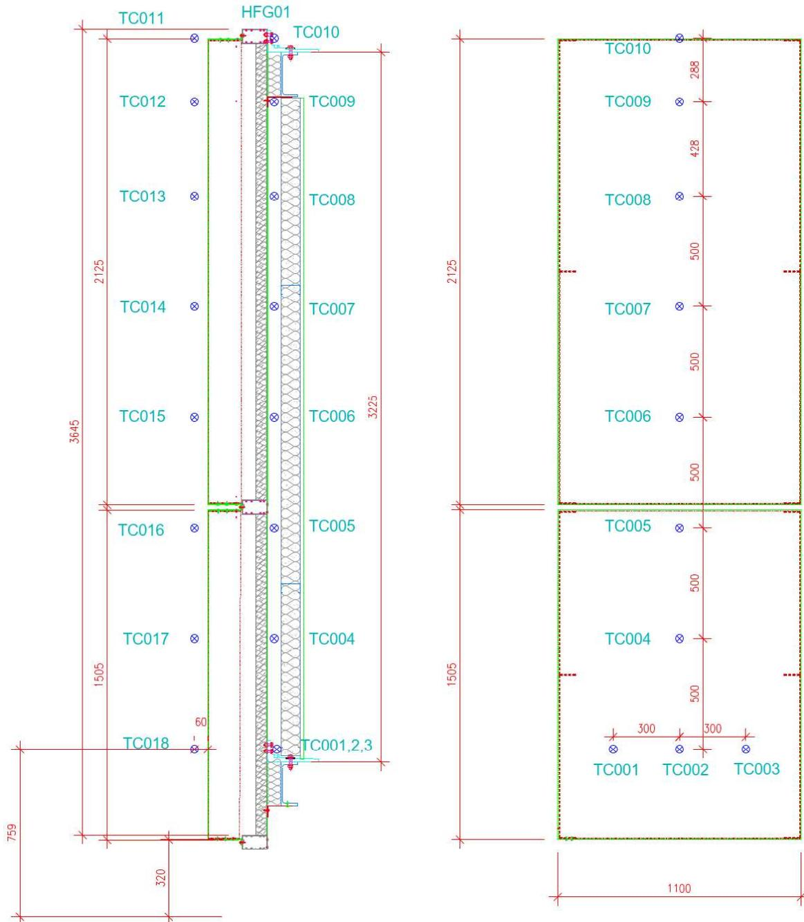
Figure 1 Instrumentation location
