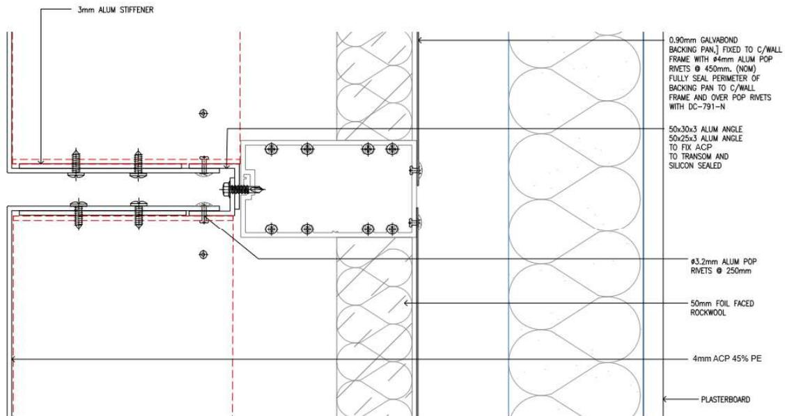
**Figure 10 System assembly – middle join detail (D05)**
