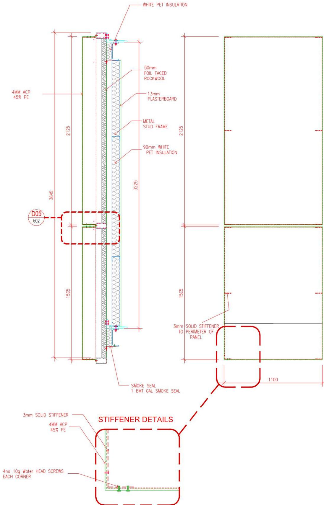
Figure 8 System assembly – Front and side view
