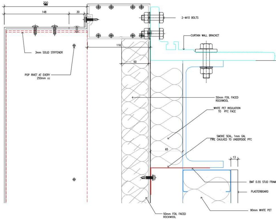
**Figure 9 System assembly – top edge detail**
