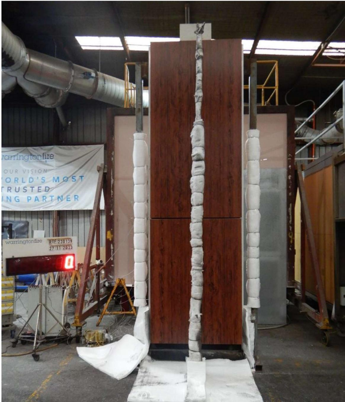
Figure 11 The specimen before the reaction to fire test
