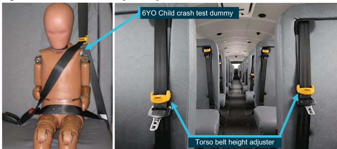
Figure 22: 6YO Child test dummy with adjusted seatbelt
