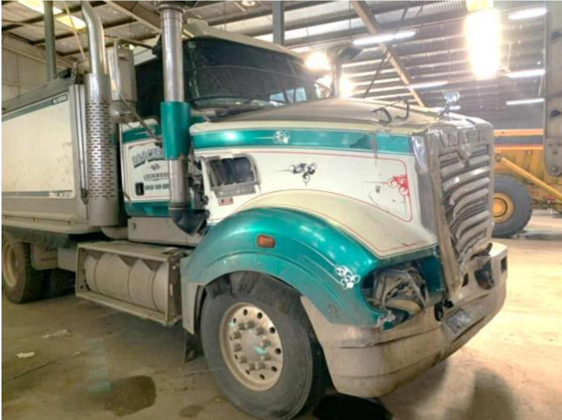
Figure 16: Mack tipper truck frontal damage
