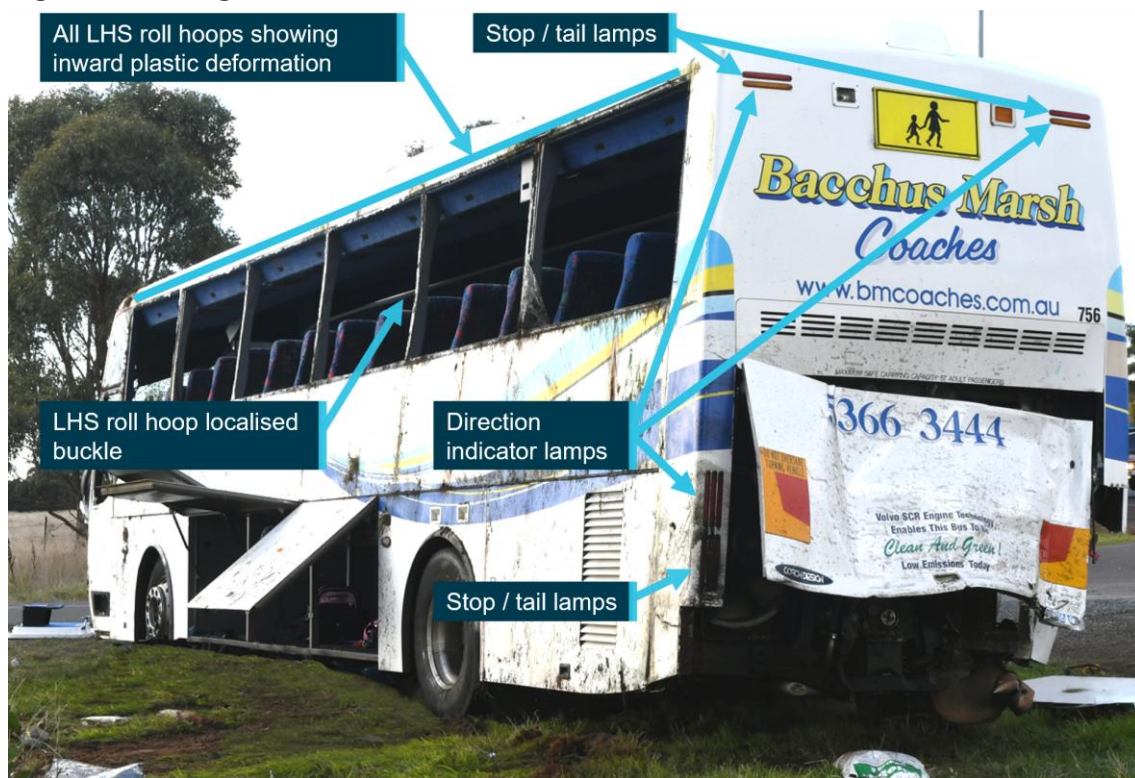
Figure 11: Damage to left side and rear of bus
